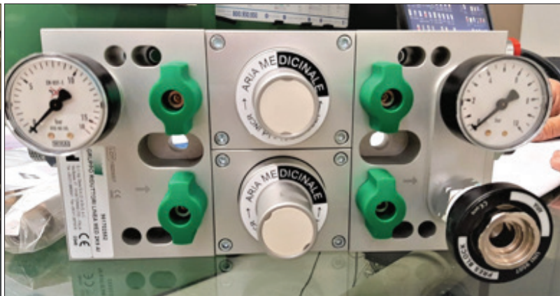
Figure 2: Medical device controlled outside the hyperbaric chamber to switch from oxygen to medical air in order to permit mask breathing for the whole HBO 2 session
