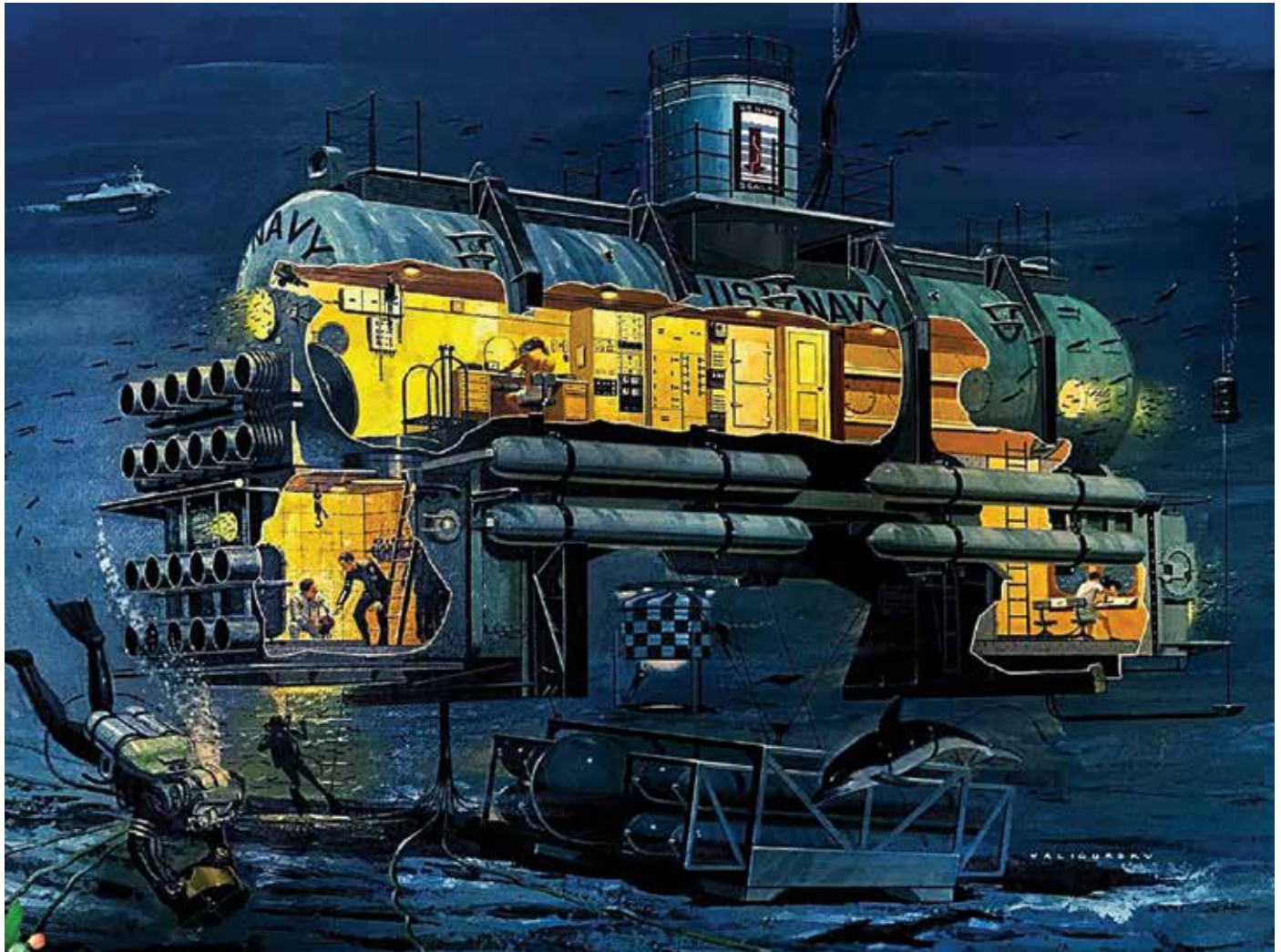
FIGURE 1: The SEALAB III habitat was a heavily modified SEALAB II structure. Two additional lower rooms were added for buoyancy and work space. The habitat floated off the seafloor to solve the “Tiltin’ Hilton” leveling problem. Legs were to be extended from the habitat to stabilize the habitat once it was level in all axes. Diver umbilical storage was added to one end. On deployment, Ballast Tanks 1 and 2, in and below the sail, were flooded at the surface. Ballast Tank 3, the large tank in the center of the ballast frame, was flooded on the seafloor. The checkerboard DIVERCON I construction project is seen in the distance. (Photo: Official U.S. Navy Illustration, courtesy of Bob Barth).
