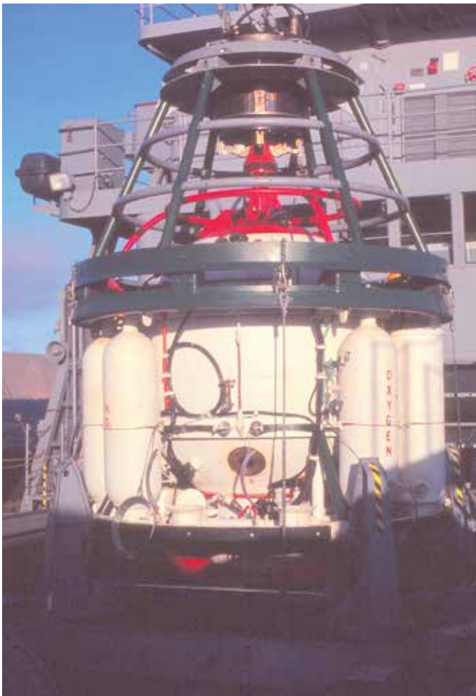
FIGURE 3. The PTC mated to the DDC. The PTC has a “lifting cage” used to manage movement of the PTC when lifted by the gantry. It remains with the ship when the PTC dives. Upon recovery, the red probe above the PTC is engaged by three latching dogs, clearly seen in this photo. (Official U.S. Navy photo)
